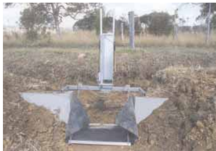
FIGURE 5.3 Padman pneumatic flood irrigation gate
