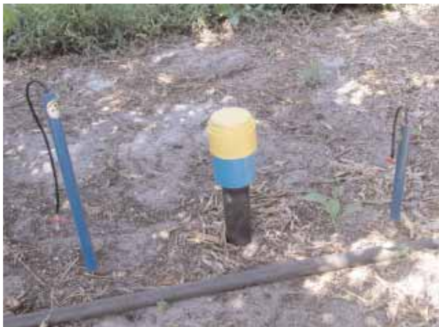
Figure 5.25 Capacitance probe with tension lysimetre.
