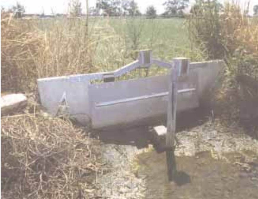
FIGURE 5.4 Automated gate with mechanical timer
