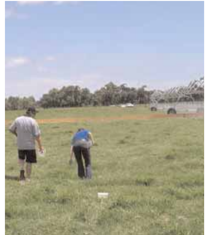
Using plastic containers to measure distribution uniformity of a centre pivot
