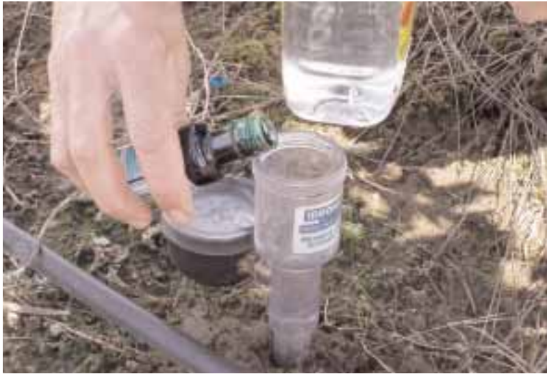
FIGURE 5.24 Adding a dye to water inside a tensiometer makes reading levels easier.
