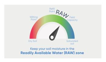
**Figure 4** A typical summed soil moisture graph reported via smartphone apps or PC platform. A summed graph is a cumulative total of all 10 cm increment sensors of the probe. 40cm probes are typical for pastures and 80cm-100cm for crops.
