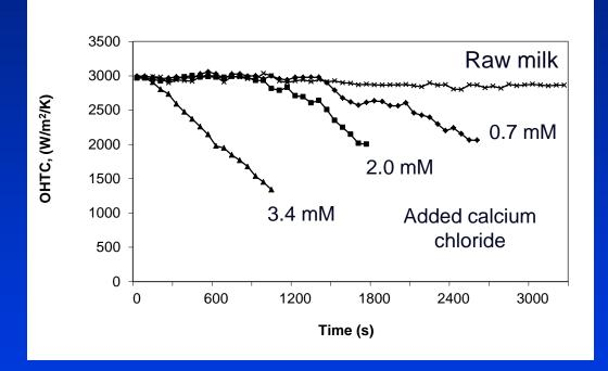
Fouling of raw cow's milk with 0 mM (x), 0.7 mM ( $\blacklozenge$ ), 2.0 mM ( $\blacksquare$ ) and 3.4 mM ( $\blacktriangle$ ) added calcium chloride during processing at 135°C for 4 s (*Note: the lower the OHTC, the more fouling*)
