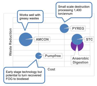
Figure 13 Mapping of sludge reduction technologies
