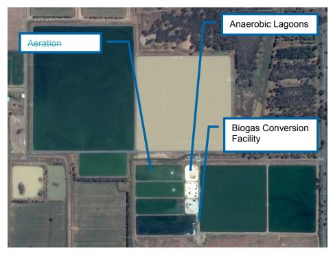
Figure 13 Aerial View of Anaerobic Systems
