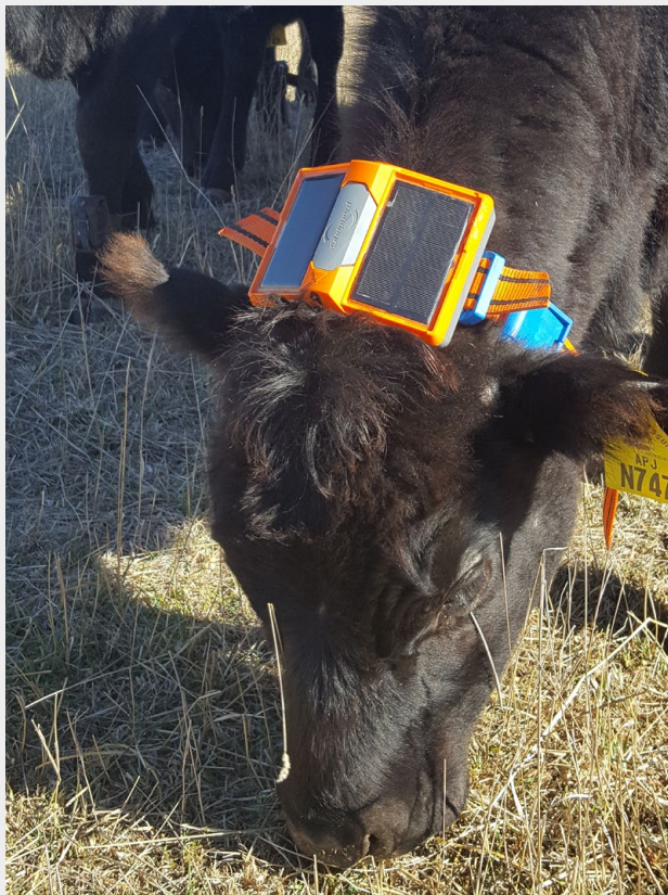
Figure 2 Photo of the pre-commercial prototype (eShepherd®, Agersens, Melbourne, Vic) that was used in many of the animal studies in the Project.
