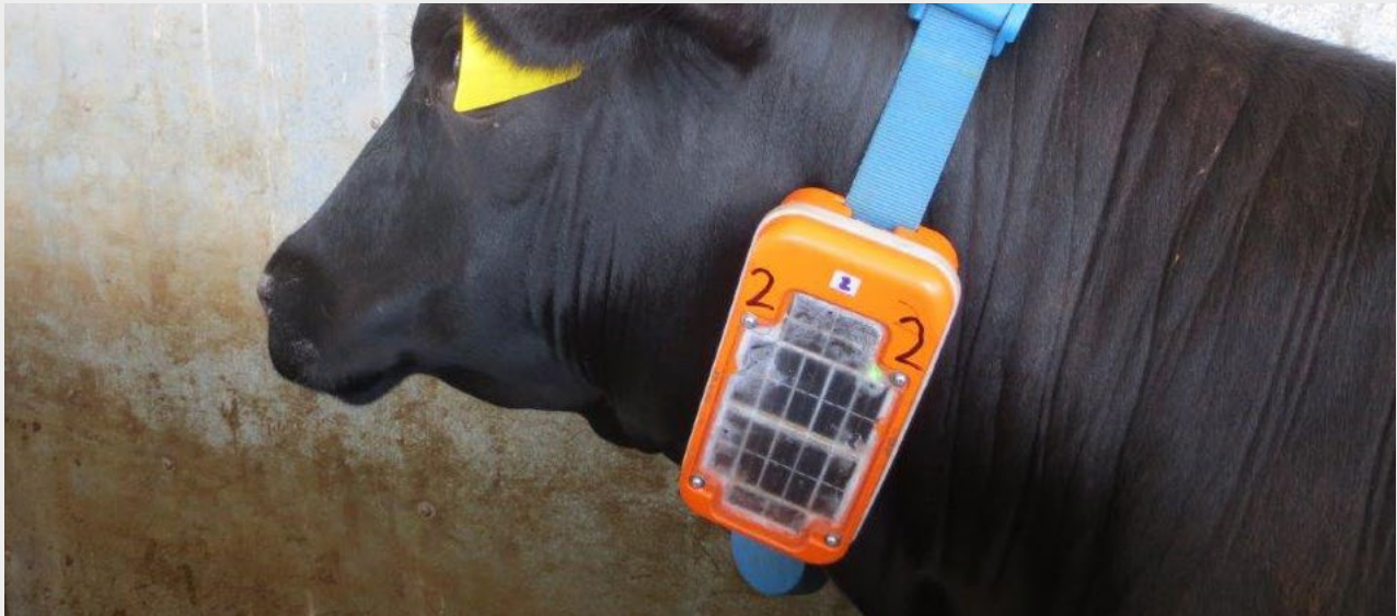
Figure 2 Photo of the pre-commercial prototype (eShepherd®, Agersens, Melbourne, Vic) that was used in many of the animal studies in the Project.
