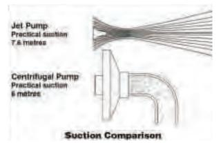
The jet pump is also versatile. By changing the venturi and jet assembly combination within the pump, the head and flow performance can be altered to suit the application.
