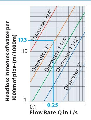
The friction chart above, shows that the nearest pipe size is 1 inch.
