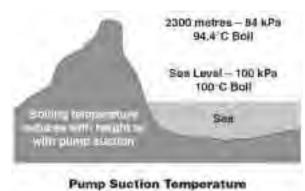
Water flowing in the suction pipe and entering the pump impeller can be extremely turbulent, releasing water vapour which can destroy the partial vacuum created by the pump.
