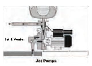
An injector containing a jet and a venturi added to the suction of a centrifugal pump increases the suction lift to between 7-8m and is known as a jet pump.
