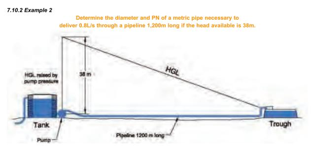
Available head is 38m, length is 1,200m, the flow rate is 0.8L/s.
