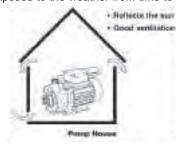
All pumps should be adequately housed to protect them from sun, weather and dust. Pump houses should be constructed to provide ventilation to the motor for cooling so the motor runs as close to air temperature as possible. There should not be any buildup of heat in the pump house and pumps should be easily accessible for servicing.
