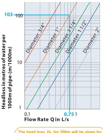
Use of the friction chart to determine head loss per 1,000m.
