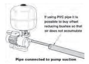
It is preferable to use an offset reducer as this keeps the top of the pipe flat and reduces the possibility of forming air pockets in pump suction.
