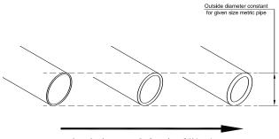
Increasing pipe pressure rating (increasing wall thickness) for metric pipe sizes
