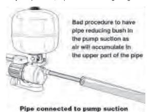
If reducing the suction pipe size at the pump, be careful not to create cavities for air pockets as this may cause the pump to lose prime when operating.
