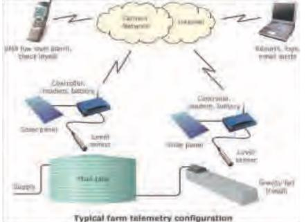
The technology selected to carry information will depend on factors such as distance, availability, type and frequency of data transmission required, and finally an analysis of fixed and variable costs.
