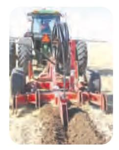
There are some disadvantages with laying pipes using rippers. It is not possible to observe the pipe in its final resting place, making it difficult to know if the pipe has been stretched as it was installed, especially when using powerful equipment. Installing the pipe at depths below 300mm can take a lot of additional work such as preripping and the use of a heavy-duty ripper driven by a powerful tractor.
