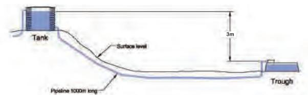
to a trough 1,000m away with a head of 3m as shown below.
