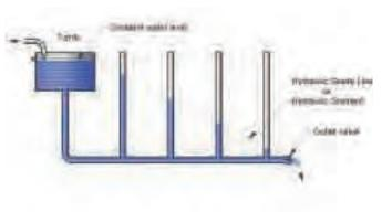
In the model shown above, a straight line can be drawn from the water surface at the tank through the water level in each clear tube to the outlet.
