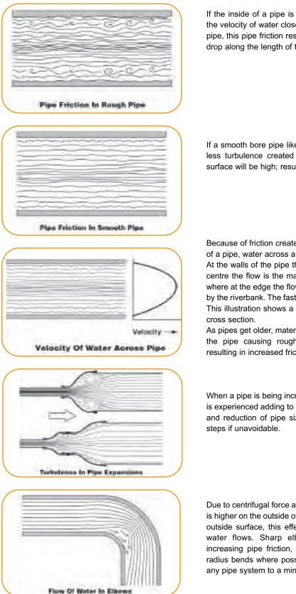
If the inside of a pipe is rough, the turbulence created restricts the velocity of water close to the pipe wall. Using a smooth bore pipe, this pipe friction results in lower flows and higher pressure drop along the length of the pipe.
