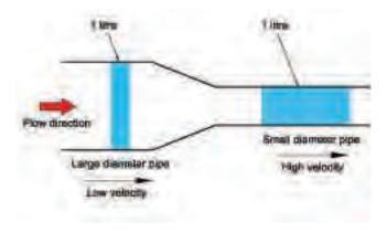
For a given flow rate the smaller the crosssectional area, the higher the velocity and therefore the higher the friction loss. 7.4 Friction loss and the hydraulic grade line
