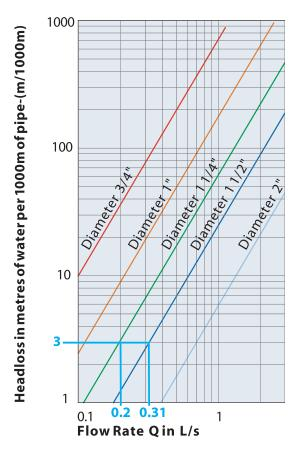
Under these conditions a  $1\frac{1}{4}^{n}$  pipe would give a flow rate very close to the required 0.2L/s. A  $1\frac{1}{2}^{n}$  pipe would give a flow rate of 0.31L/s.
