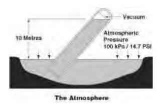
If this same tube is laid on an angle and again creating a perfect vacuum within, the atmospheric pressure would again push the water up the tube to a height of 10m.
