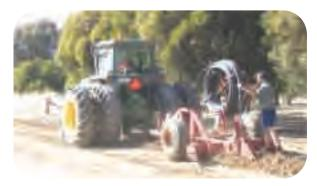
There are a number of commercially-available pipe rippers with various features such as spinners (to hold the pipe coil) to avoid manual feeding of the pipe. The coil still needs to be manually lifted into the spinner.
