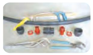
1. The tools required to mend a damaged Imperial pipe or to join two Imperial pipe ends are: a hacksaw, small knife or preferably pipe cutters, block of wood, a joiner.
