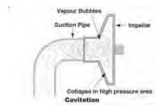
The vapour bubbles causing cavitation reduce the efficiency of the pump and can cause pitting and erosion of the impeller or casing of the pump.
