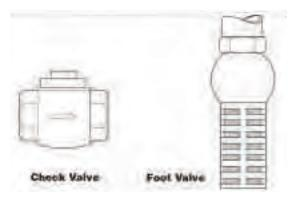
The check valve is also known as a one-way or non-return valve. The sole function of this valve is to stop any reverse flow.
