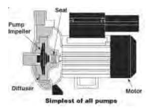
Centrifugal pumps are efficient, simple to maintain and are one of the most common pumps available.
