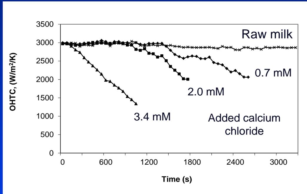
Fouling of raw cow's milk with 0 mM (x), 0.7 mM (◆), 2.0 mM (■) and 3.4 mM (▲) added calcium chloride during processing at 135°C for 4 s
