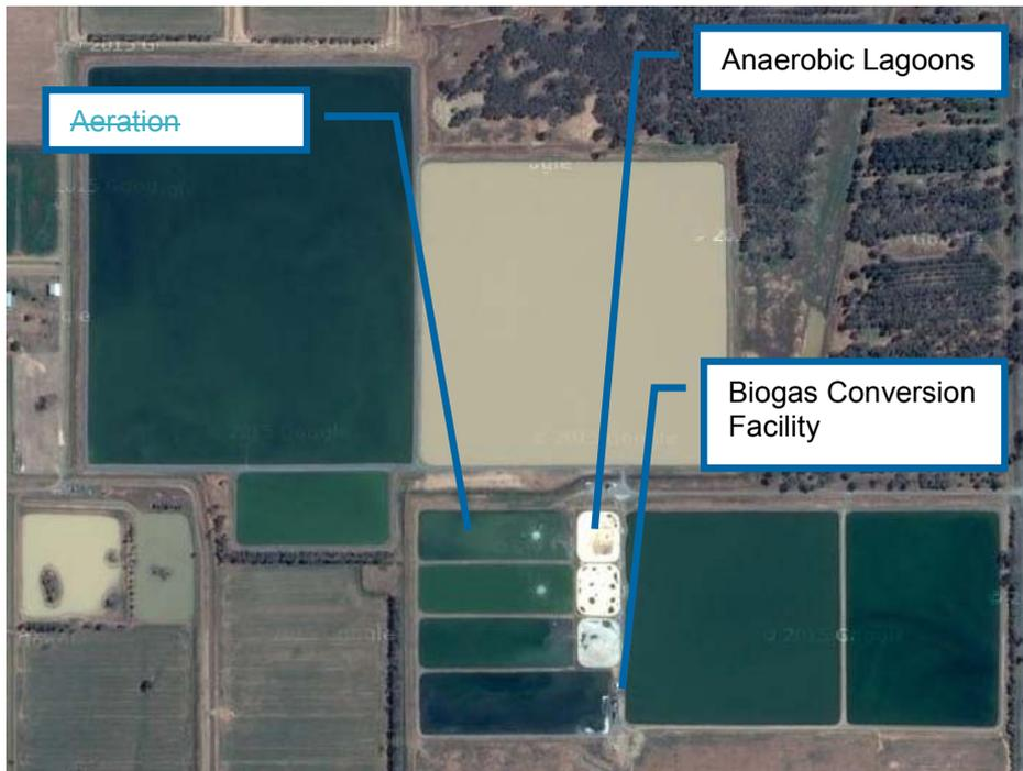
Figure 13 Aerial View of Anaerobic Systems
