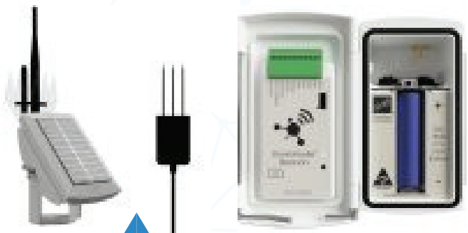
Example of EnviroNode sensor and beacon with solar panel
