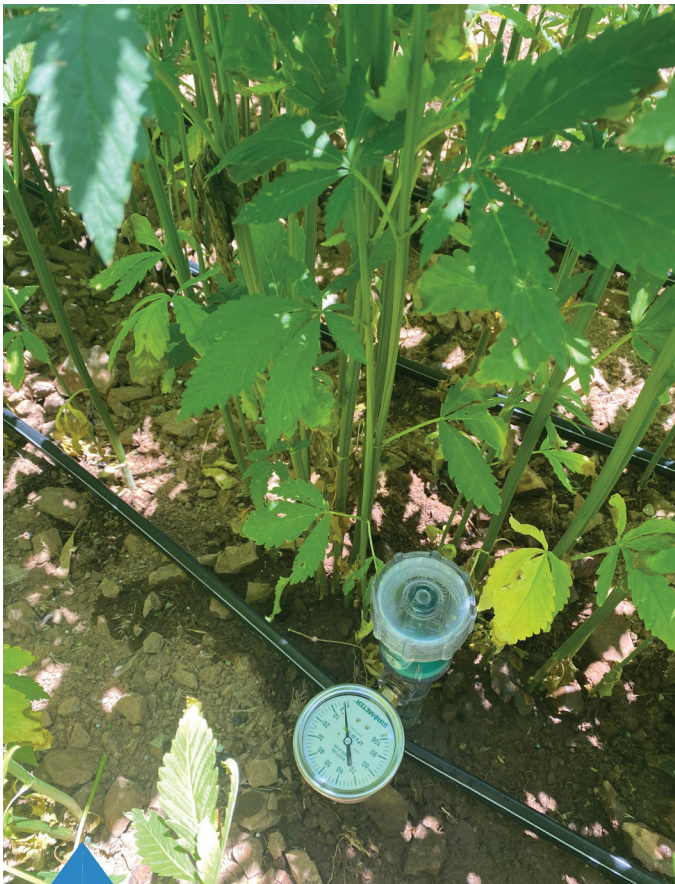
Example of tensiometer installed in field of industrial hemp
