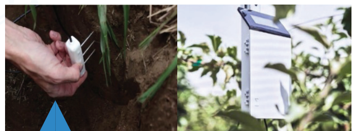
Decagon TEROS-12 soil probe and ZL6 data logger in field Image: https://edaphic.com.au
