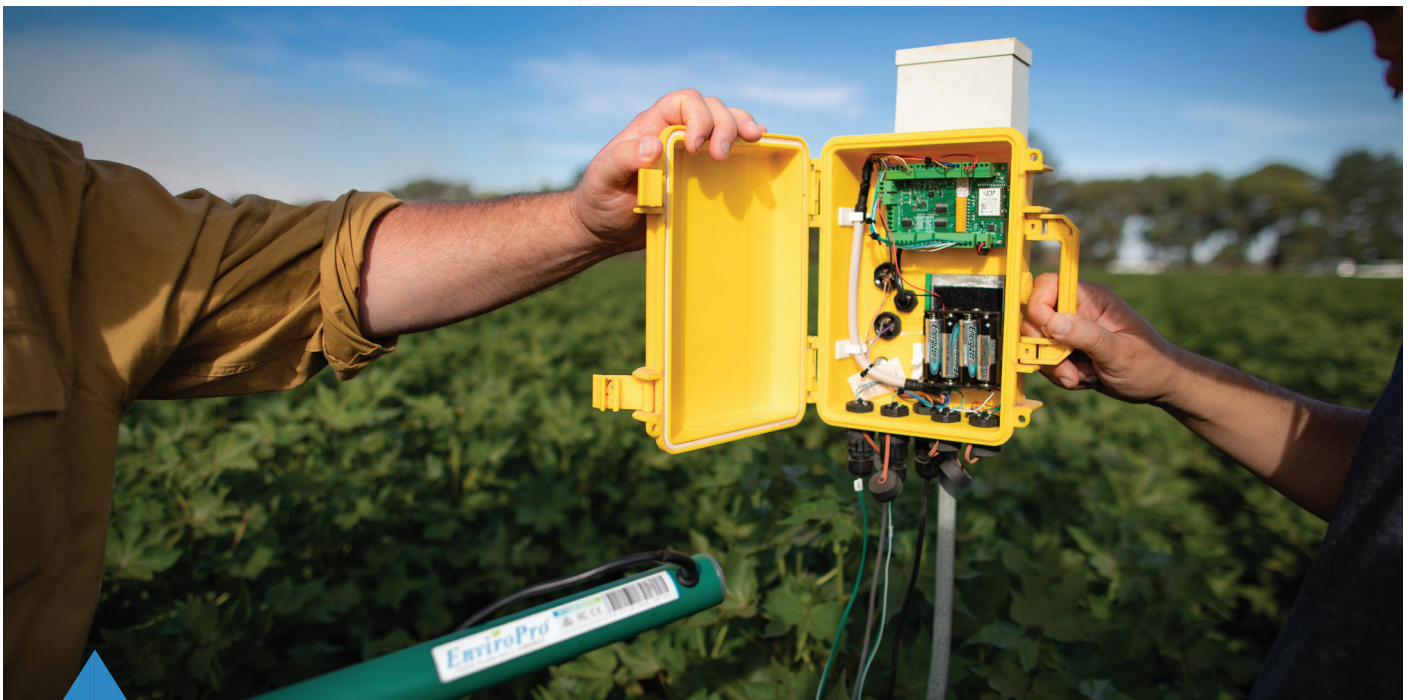
Capacitance Soil moisture probe with telemetry and data logger
