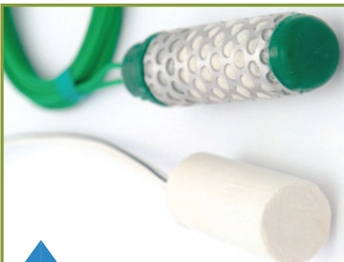
Example of Granular Matrix sensor (top) and Gypsum Block (bottom)
