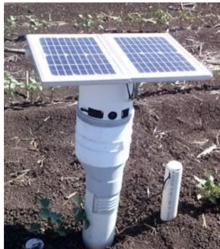
Vertical installation of MP406 sensors installed at three depths, with access tubes.
