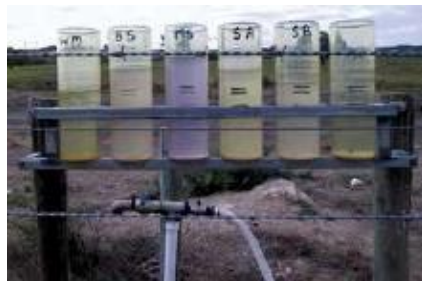
IRRIGAUGEs installed and numbered to match watering sections. The black lines mark the irrigation point for summer and autumn/spring.
