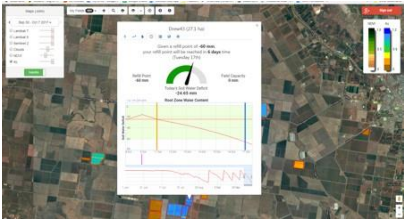
IrriSAT screenshot showing the irrigation scheduling tool component that shows previous and forecasted crop water use and estimated time to next irrigation.
