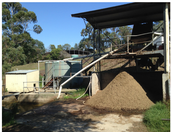
Figure 11. Separating liquid and solid manure fractions using a sieve and mechanical screw-press.
