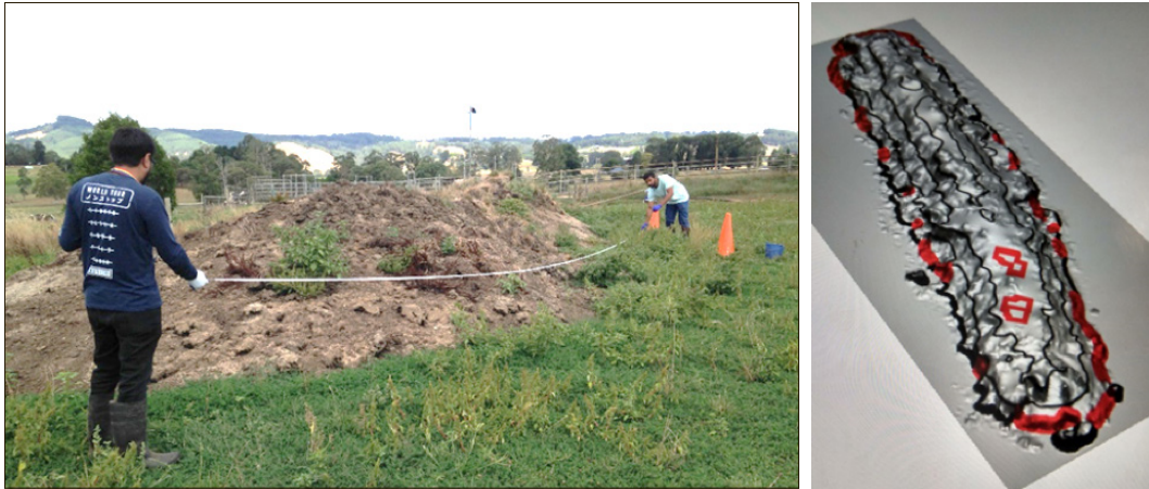
Figure 12. Determining volumes of manure stockpiles.
