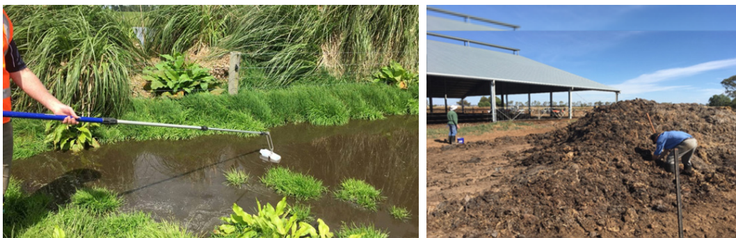
Figure 13. Collecting a representative sample of pond or stockpiled manure for laboratory analysis.
