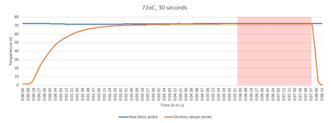
Figure 10. Temperature read out from the data logger files for the pasteurisation experiment. The blue line represents the temperature of the heat block, and the orange line represents the temperature of the dummy milk sample. The red box represents the period of time where the dummy sample reached the appropriate temperature, and spiking experiments were conducted in this time period.
