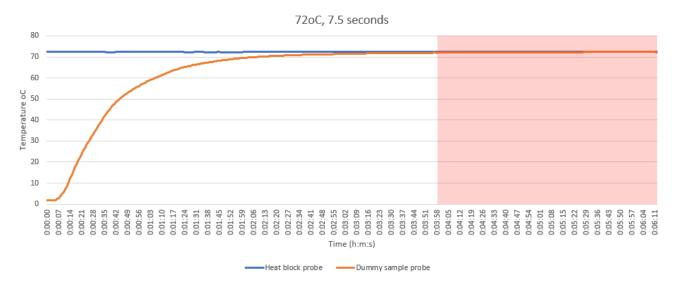
Figure 2. Temperature read out from the data logger files for the pasteurisation experiment. The blue line represents the temperature of the heat block, and the orange line represents the temperature of the dummy milk sample. The red box represents the period of time where the dummy sample reached the appropriate temperature, and spiking experiments were conducted in this time period.
