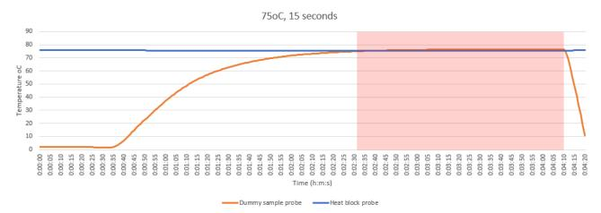
Figure 18. Temperature read out from the data logger files for the pasteurisation experiment. The blue line represents the temperature of the heat block, and the orange line represents the temperature of the dummy milk sample. The red box represents the period of time where the dummy sample reached the appropriate temperature, and spiking experiments were conducted in this time period.
