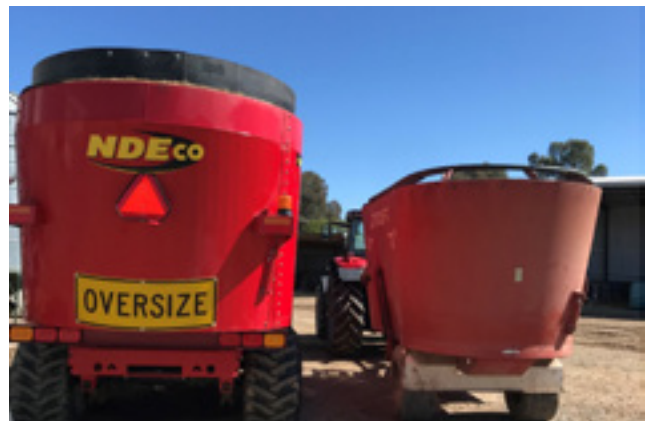
The new 28m 3 mixer wagon next to the older 15m 3 mixer wagon
