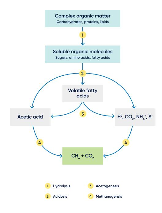
Note: Hydrogen =  $H^2$ , Carbon Dioxide =  $CO_2$ , Ammonium =  $NH_4^+$ , Sulphide =  $S^-$ , Methane =  $CH_4$ Source: Adapted from Hamilton, 2017
