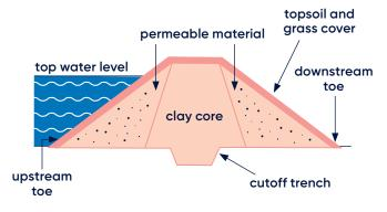
**Figure 4.** Common embankment core construction method – typical upstream clay core
