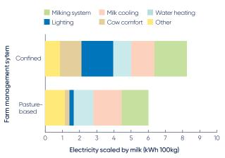
Note: Confined = Contained. Electricity use in kWh per 100kg milk broken down into the component of the dairy operation the energy is used in.
