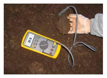
C: Example of compost that is too dry with insufficient temperature – will not form ball
