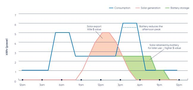
Figure 106. Graph of energy consumption and solar generation in a typical dairy
