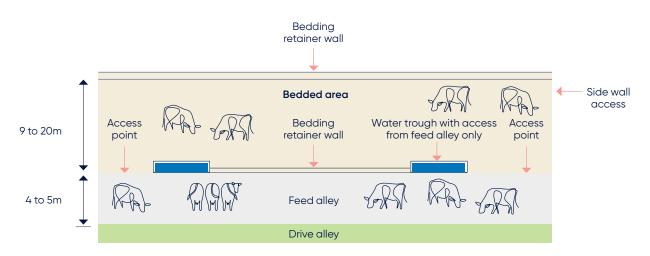
Figure 35. Concrete retaining walls provide separation between the feed alley and the bedded pack area which is helpful in managing pack moisture
