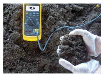
B: Example of compost that is too wet with insufficient temperature – forms firm ball with water drops
