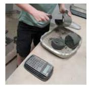
The Proctor Compaction Test, to find the range of moisture contents over which the required level of compaction can be achieved.
