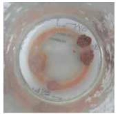
The Emerson Aggregate Test, to see how dispersive or prone to erosion the soil is.
