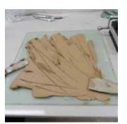
The Atterberg Test, determines the clay's plasticity.
