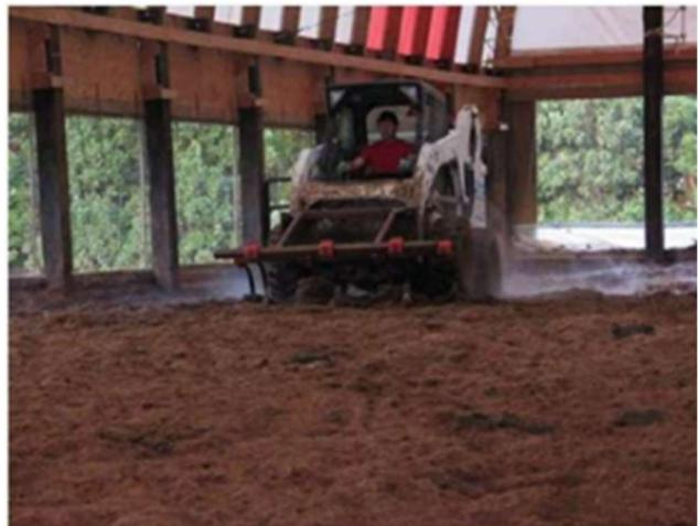
Figure 14. Compost darn, bedding pack being tilled (15)
