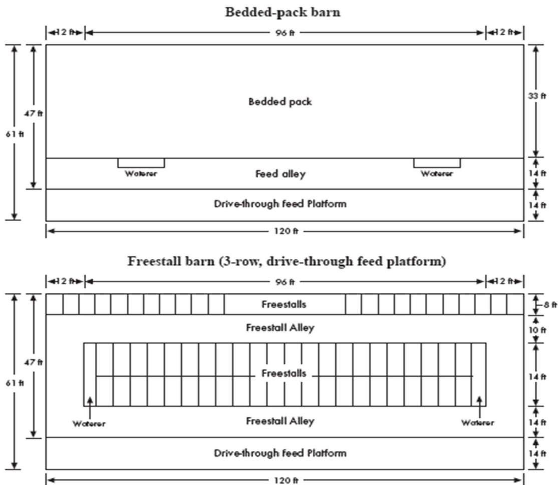
Figure 5. Cow capacity of free-stall (78 cows) and composing bedding barns (39 cows) with the same footprint. Source. Gay, S. W., *Bedded-pack Dairy Barns* (32)
