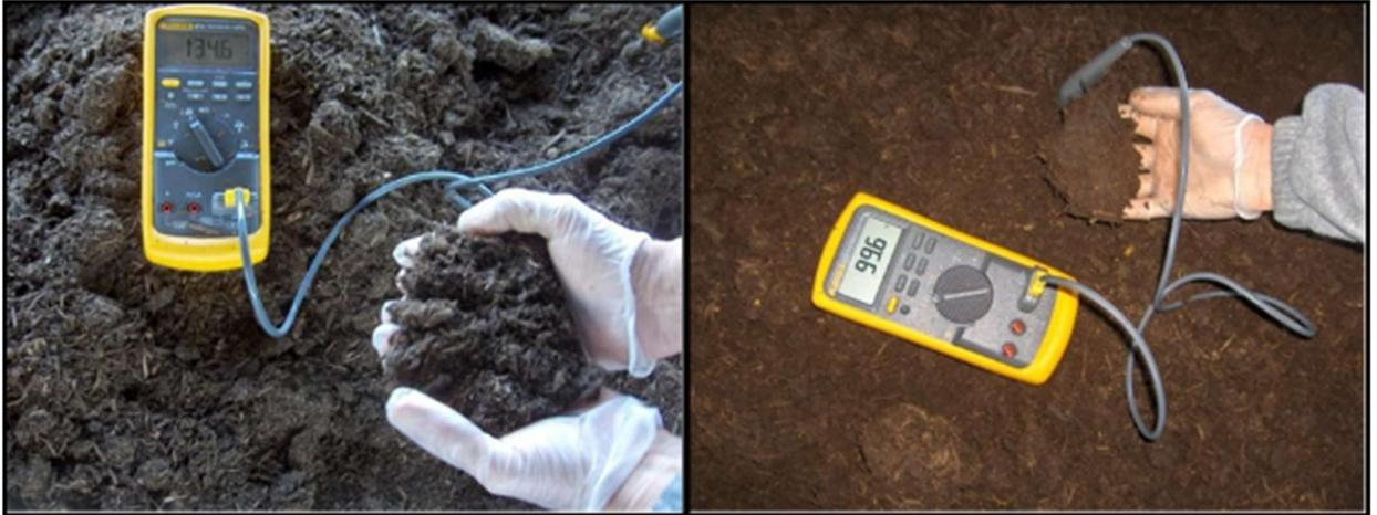
**Figure 19. Examples of compost-bedded packs of various temperatures. Light and fluffy compost with ideal temperature of 134.6 °F (57°C) is shown at left. Wet and chunky compost with below-optimal temperature 99.6 °F (37.5°C) is shown at right. Source Bewley et al (Ref. 17)**
