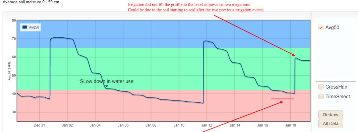
Average moisture chart of the 50cm profile at flood irrigation site under corn
