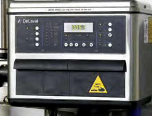
Figure 5 A semi-automatic wash controller for a bulk milk vat (example only)
