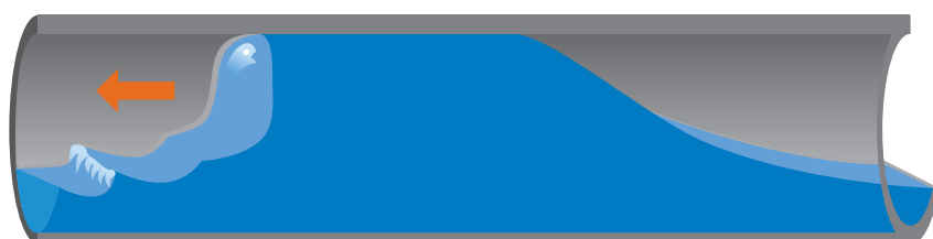
Figure 25 A well-formed slug in the milk line
