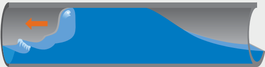
Figure 38 A well-formed slug in the milk line
