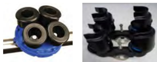
Figure 7 Two types of jetters: the one on the right provides support to the cluster
