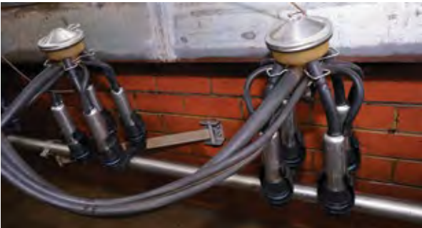
Figure 9 Clusters attached to jetters mounted on the jetter line in the cleaning position (example only). Two different cluster orientations when attached to the jetters are shown
